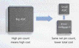
Instead of using a costly high pin-count ASIC, use the same ASIC design in a smaller package—plus an inexpensive Xilinx CPLD—and get the same I/O, but at a much lower cost.
